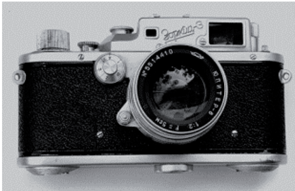
Fig. 19. Zorki 3, full range of speeds via two dials.
