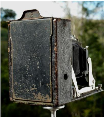
*Pic 14. The very small, thin metal single plate holder with numbered dark slide.*
