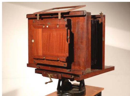
*Pic 2. Reducing back and focus frame (minus ground glass) - note the rear focus crank which racks the front standard back and forth.*
