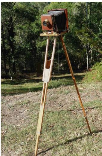
**Pic 9.** Original tripod (third leg obscured) cleverly fitted into camera base.
