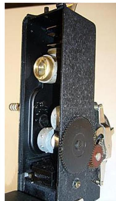
*Rear section, with lamp holder and drive sprocket visible.*
