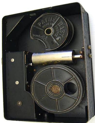
*The SCREENUS, showing the film chamber, reels and lamp holder. (Projection accessories shown: Reels and lamp holder are removed and a Pathé style camera film cassette inserted for camera use.*
