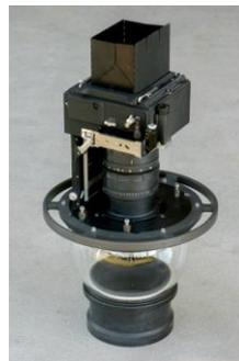
The APCS has been asked by a PHSNE Member to advertise this one-of-a-kind 360 degree lens mounted to a Graflex 5x4 Press Camera – produced in the early 1960's by Space Optics Research Labs, New Hampshire, specifically to capture a 360-degree image from a high vantage point, eg from an aircraft, a balloon, etc.
