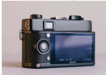
Ollie removed the back door of the camera, modified the chassis of the camera so sensor would fit in the film plane, and used a 3D printer to print a new back cover to hold the workings.
