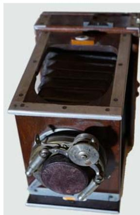
A JP Shew “XIT” strut from 1898. This one is fitted with a Dallmeyer 5-element lens on a B&L shutter that is clearly a Shew modification. The camera comes with half a dozen original dark slides.
