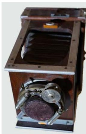
A JP Shew "XIT" strut from 1898. This one is fitted with a Dallmeyer 5-element lens on a B&L shutter that is clearly a Shew modification. Some research has identified the lens in the stock books from Dallmeyer and supports the manufacture date. The camera comes with eight original dark slides.
