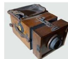
A JP Shew "XIT" strut from 1898. This one is fitted with another very advanced lens, a Dallmeyer 5-element lens on a B&L shutter that is clearly a Shew modification. Some research has found the lens in the stock books from Dallmeyer for 1898. The camera comes with eight original dark slides.
