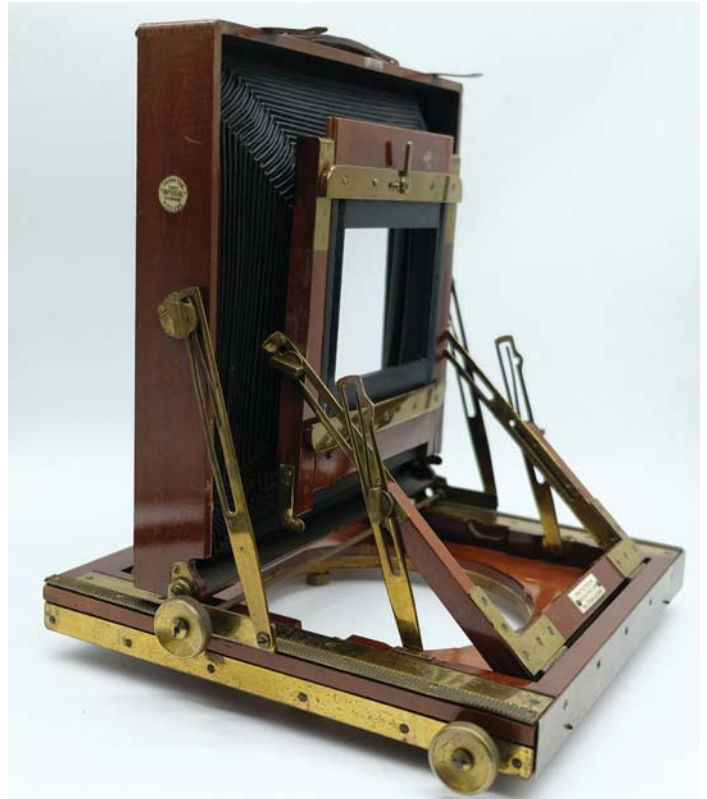
The triple extension is commonly pictured in the extended form - 600mm ie 3 times the length of the base. This view is in the extreme wide angle position. Adjusting those struts takes a bit of care.
