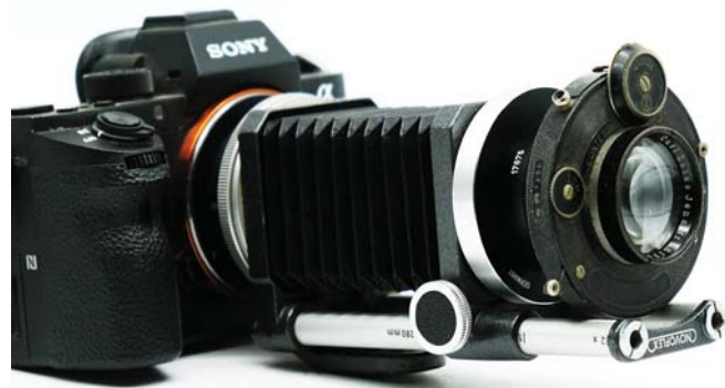
A test setup with a 135mm Tessar from the 1920s fitted to a Sony A7R using a Novoflex bellows unit and a couple of fabricated adapters
