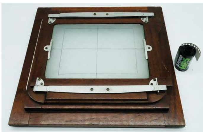
The fabricated half-plate back based on an Eastman back from around 1905 that was fitted to the candidate full plate camera.
