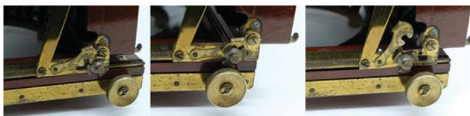
An unusual swing back adjustment on the candidate full plate camera.
