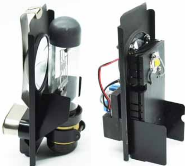
Left: the original P28 lamp assembly from a Prado, and Right, the XHP70.2 chip unit with the regulator - all mounted on a salvaged Prado plate, and the astute will note that the two plates shown here are from slightly different models. (Late Prado 500 on the left and an early 300 on the right).
