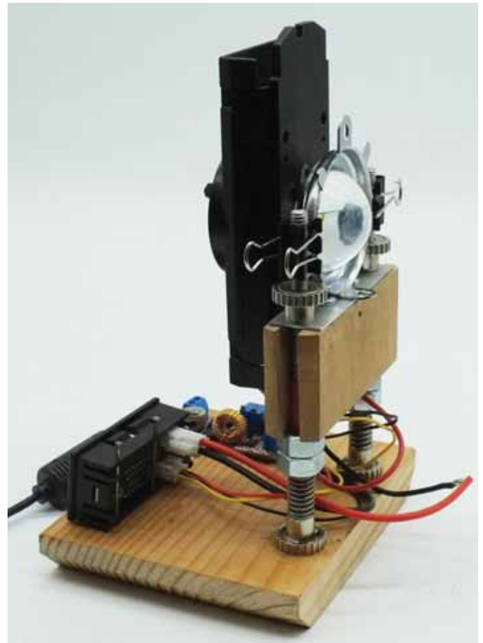
The completed lamp unit that was used in the LAVERNE magic lantern. This is clearly an experimental version and needs a bit of “tidying up”. The metering unit on the left is not essential. This version is far from unique, but provides for X, Y, and Z alignment. High voltage options exist too but with significantly increased safety risks.
